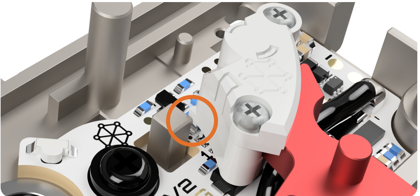
Magnet holder has to rest on the contact stopper
